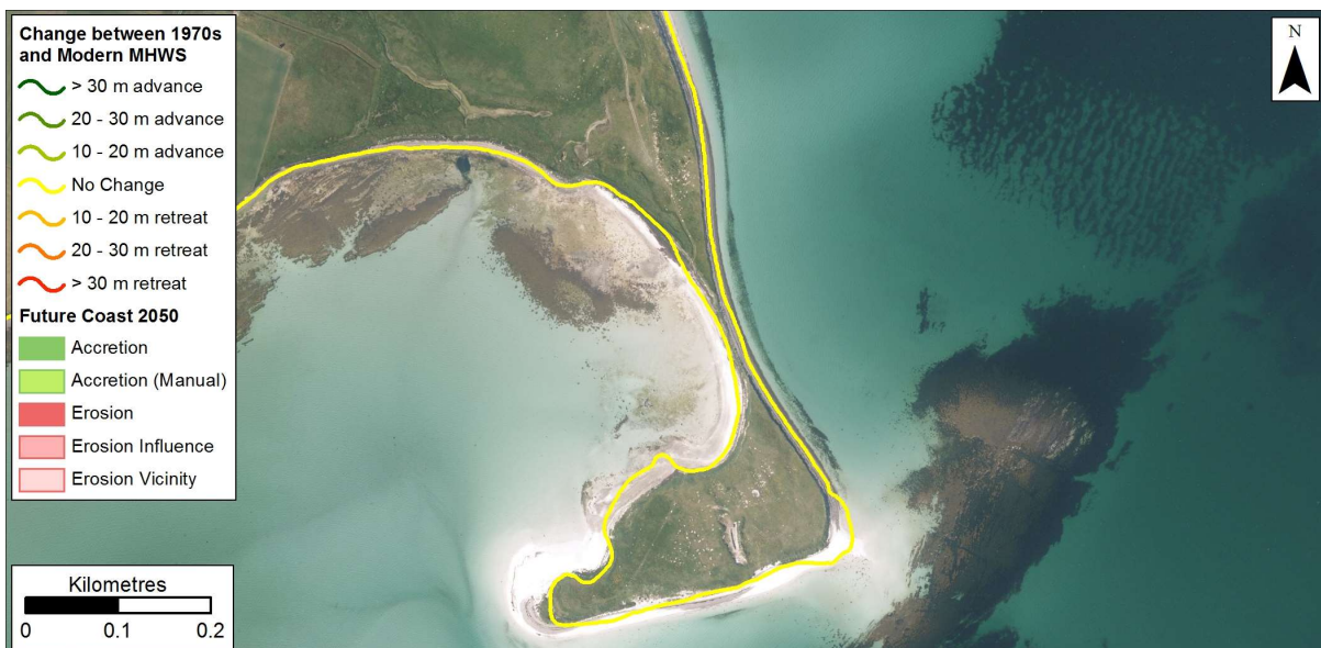
Figure 10.48: Possible future coastline position in 2050 based on rates between 1970 and Modern MHWS data at Otterswick. Getmapping are our current providers of Scotland-wide digital aerial imagery© Getmapping plc.
